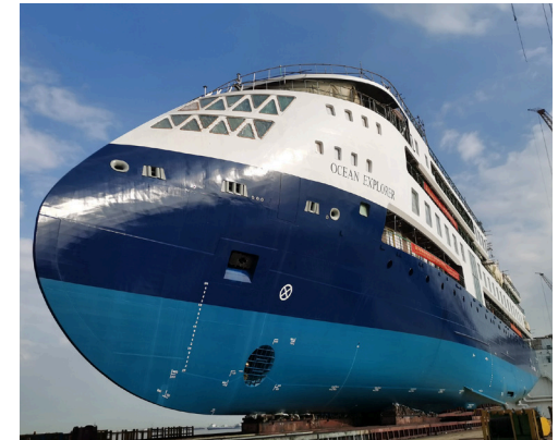
The 'Ocean Explorer' being launched - one in a series of X-BOW® expedition cruise ships under construction in China.
